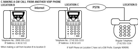
When making a call from location B to location D VoIP Phone on Location C must set GW enabled We can set IP address of Location C to shortcut dial from  $\pm 1 - \pm 5$ We can simply set this up to  $\pm 1$  with IP 4.38.32.233 While VoIP Phone's GW (Gateway) is "ON" at Location C it field Dense on Location C does not have GW encourage
